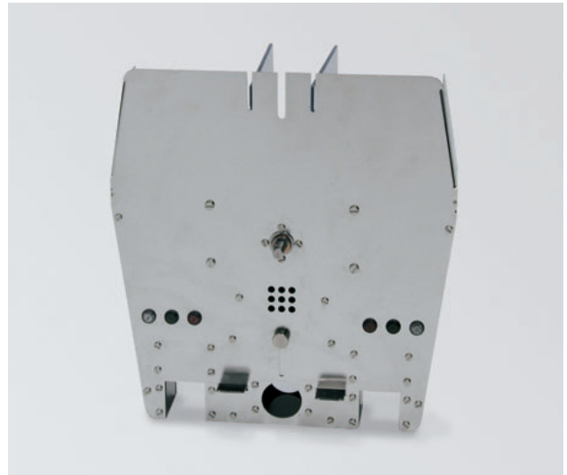
■ Operant wall with two automatic doors, two levers, stimulus lights and loud-speaker
