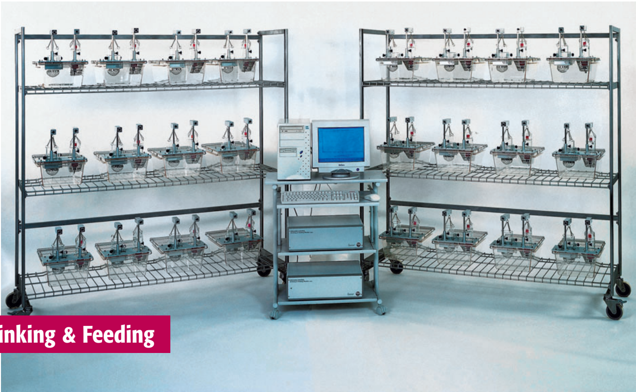
■ Standard drinking & feeding monitoring system – 24-place system
