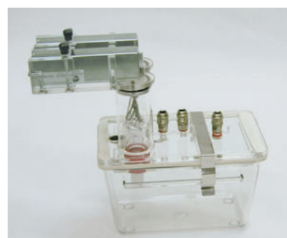
■ Calorimetry cage for mice with D & F stations
